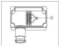
• Terminal block is located inside of the product. Unscrew the 4 bolts located in the upper body to get rid of the upper lighting element of the unit.
