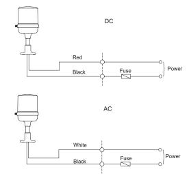
• External power line - UL2464 AWG18(0.75sq) 400mm
