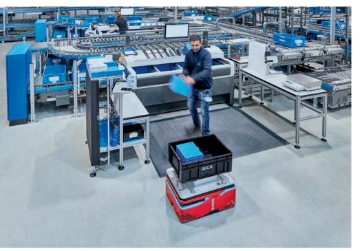
The nanoScan3 has been designed specifically for use in small mobile platforms.
