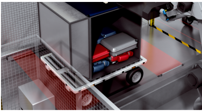
Determining the position of the baggage cart in the robot cell
