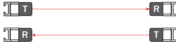
Figure 9: Light grid installed in opposite directions R = Receiver; T = Transmitter (sender)
