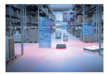
The microScan3 safety laser scanner, for example, which relies on the innovative safeHDDM® scanning technology, can be used here. It not only delivers highly precise measurement data, but is also resistant to dust and ambient light. This has a direct positive effect on the availability and productivity of the automated guided vehicle systems.
