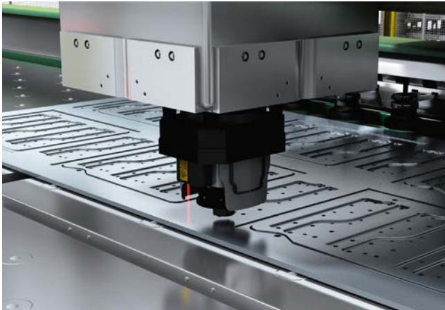
Figure 11: Checking distance at the cutter head with the OD Max displacement sensor
