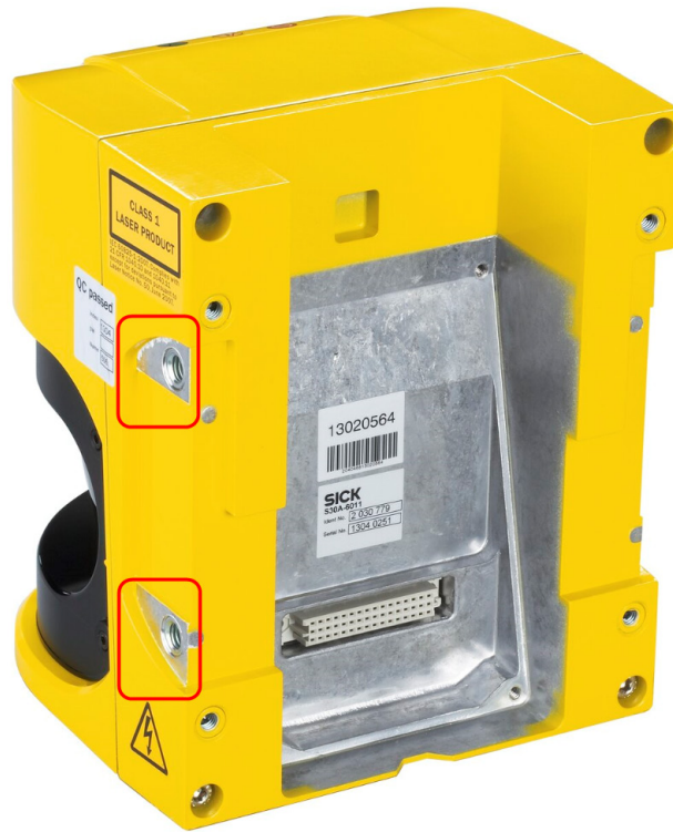
Figure 25: Possible method of connecting the functional earth
