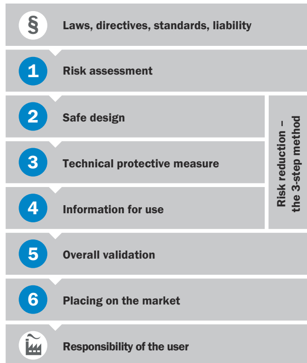
Figure 2: Structure: “Six steps to a safe machine”
