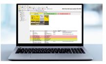
**Direct comparison in the project** The "Project comparison" function compares the configuration of the Flexi Soft safety controller with the configuration in the software. Differences and changes are visualized quickly.
