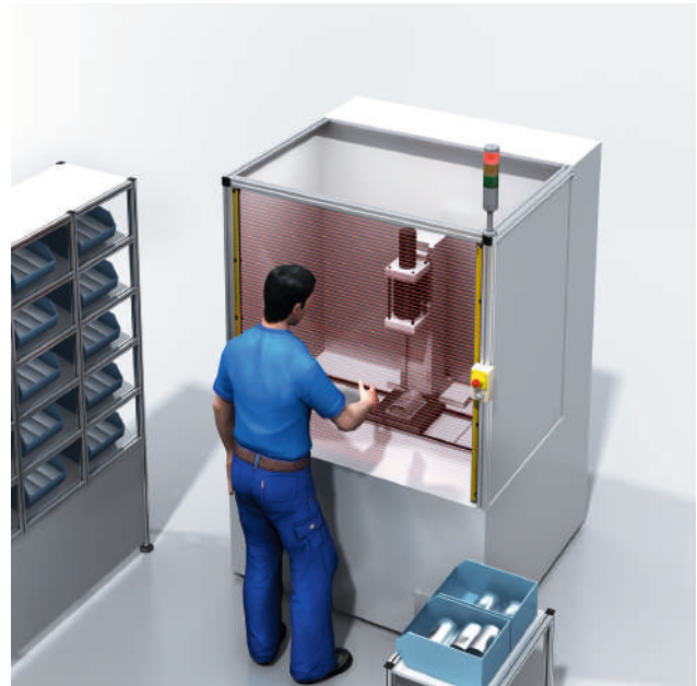
Figure 54: Hazardous point protection on an automatic assembly machine with safety light curtain
