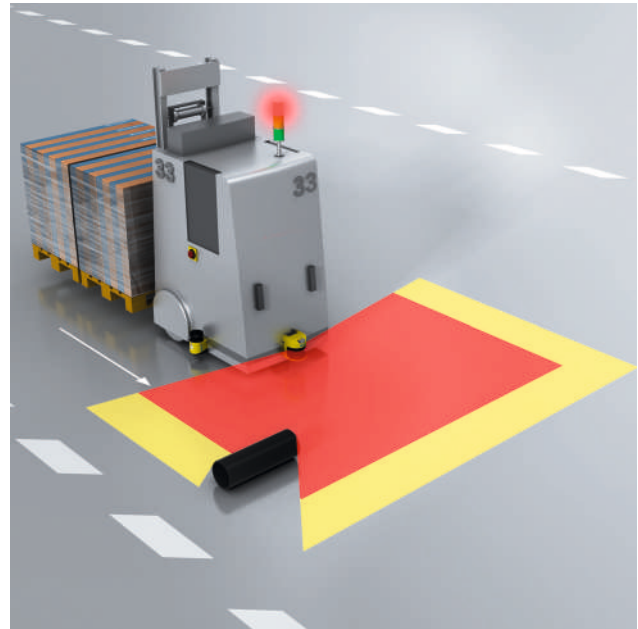
Figure 81: Positioning of a test body on an autonomous vehicle for testing the detection of a person lying down
