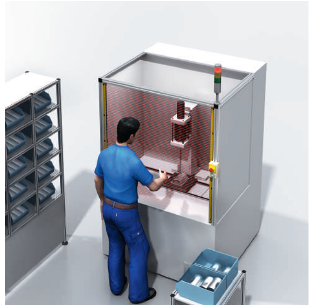
Figure 45: Hazardous point protection using a safety light curtain
