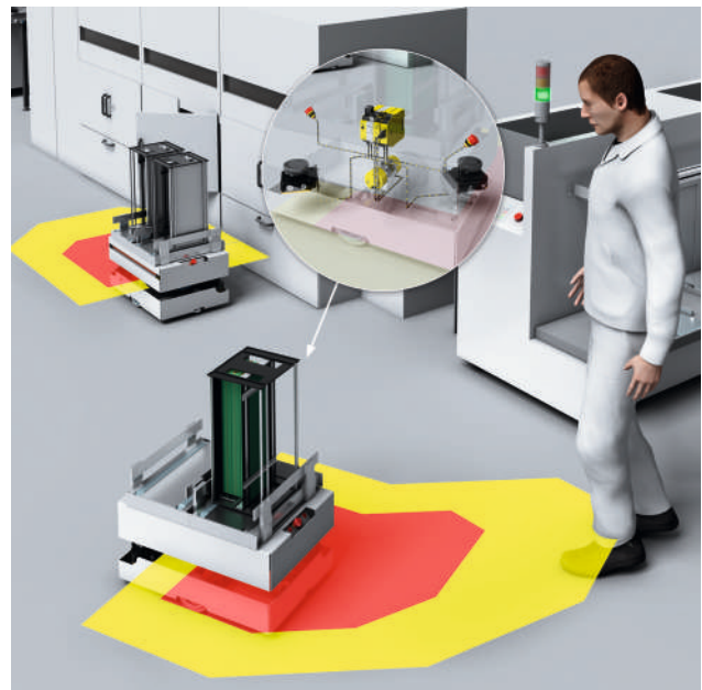
Figure 65: Application example for protective fields on an autonomous vehicle
