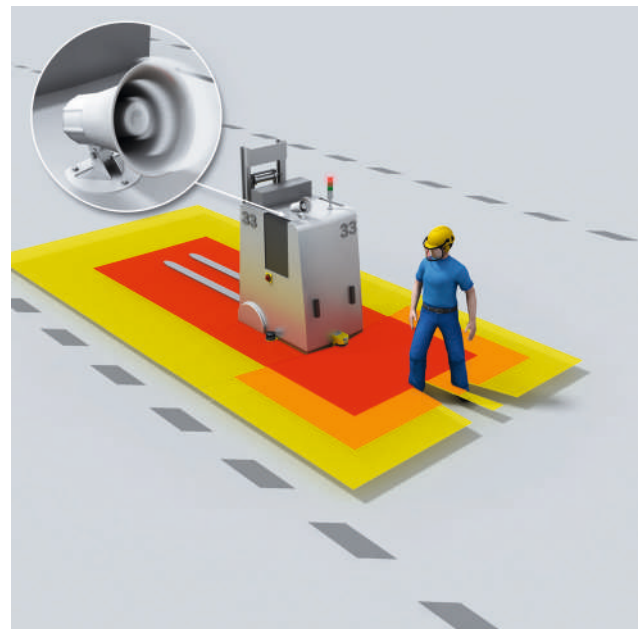
Figure 122: Autonomous vehicle with a safety laser scanner as a protective device and acoustic and optical warning device
