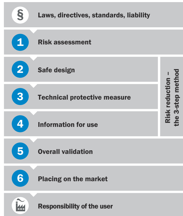
Figure 2: Structure: “Six steps to a safe machine”
