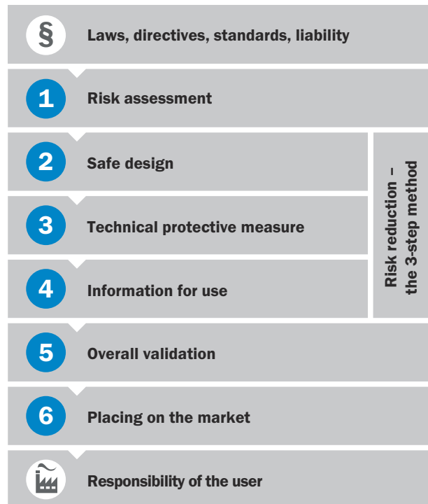
Figure 2: Structure: “Six steps to a safe machine”
