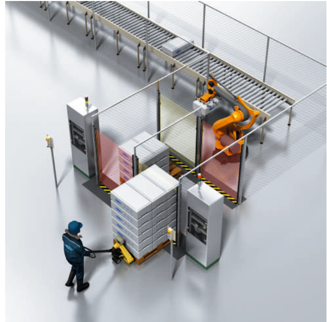
Figure 28: Safeguarding a shared work area for humans and robots using safety light curtains
