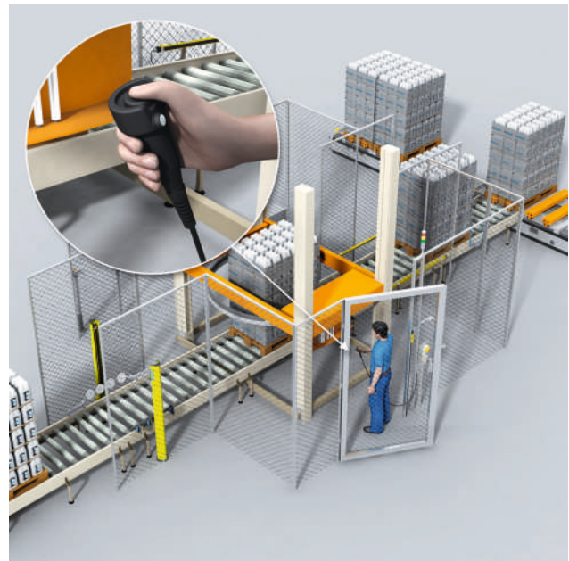
Figure 29: Safe changing of the film roll on a stretch film wrapper with the movable guard (door) open through a combination of enabling switch and safely reduced speed
