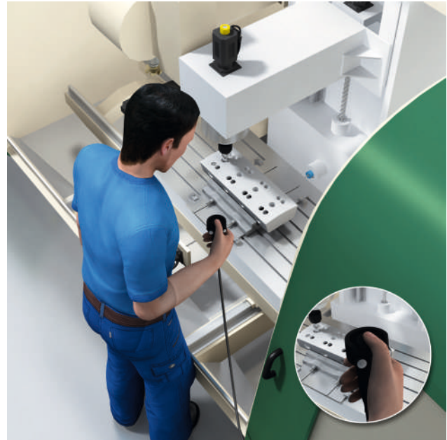
Figure 69: Enabling device for setting up an automatic drilling machine
