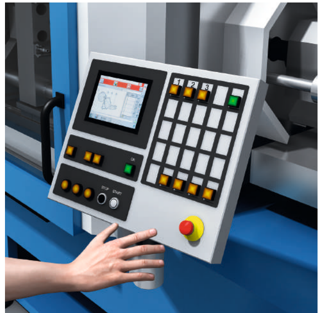
Figure 31: Emergency stop by means of an emergency stop pushbutton
