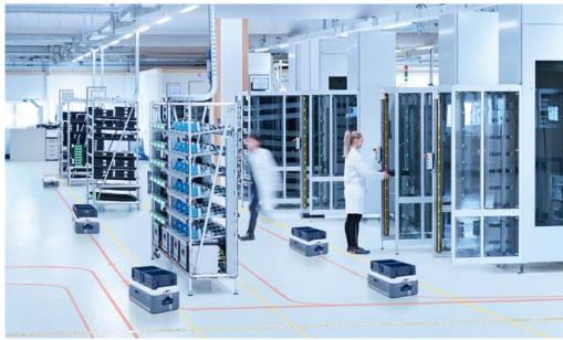
Besides small vehicles, larger AGVs (automated guided vehicles) can also optimally support automated production processes. In particular when combined with other safety sensors, for example safety laser scanners, scanGrid2 provides a tailored and economically attractive solution for protecting AGVs.
