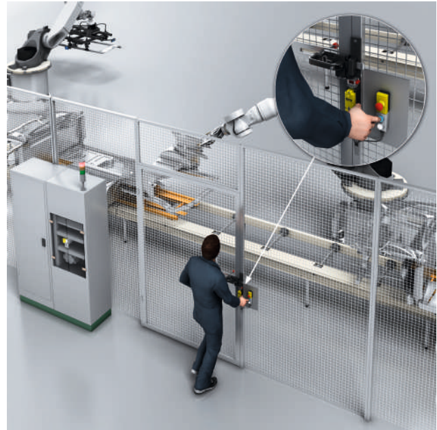
Figure 92: The position of the reset pushbutton allows a full view of the hazardous area when resetting the protective device.
