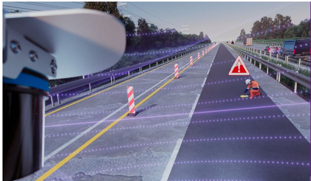
Figure 3: How distance measurement and collision avoidance works – example for road roller
