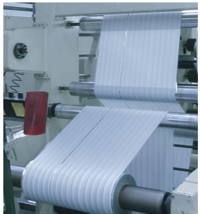
The roll is kept under tension, which allows the machine to be restarted without problems. This improves productivity.
