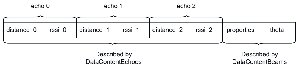
Figure 10: Example representation of a beam as a tuple. There are three echoes available. Both distance and RSSI values exist per echo, i.e., the corresponding bits of DataContentEcho have the value 1. Values for beam properties and azimuth angle are also available, i.e., the corresponding bits of DataContentBeams have the value 1.
