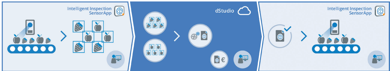
Fig. 3: A typical workflow starting with collection of the raw data by the sensor using a SensorApp, the training takes place in the cloud service and the trained Deep Neural Network is finally uploaded to the sensor again to be used to directly classify images in the factory.
