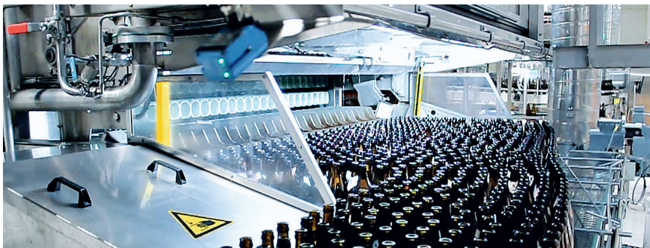
Fig. 2: Object classification is one example of a machine vision recognition task. In this user case, new and used bottles are classified in the infeed zone at the bottle-washer machine.
