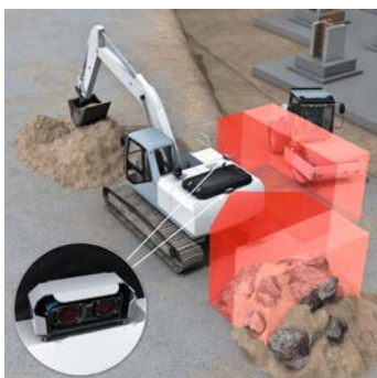
Figure 11: Stereo for active collision-warning in harsh outdoor environments
