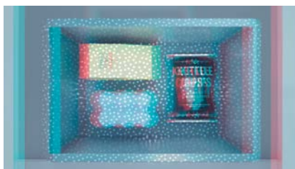
Figure 7: Step two: Overlay and correlation of left and right image enhanced by using the pattern of the non-visible structured infrared illumination.
