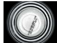
No glares, revealing print on a metallic surface.
