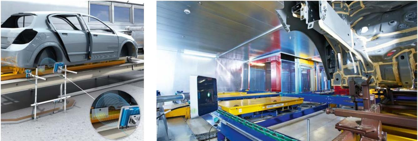
Figure 1: Car body identification with RFU630 UHF write/read device and temperature-resistant UHF label attached directly to the body
