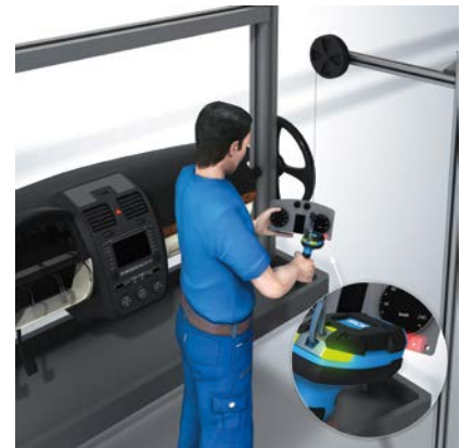
Mobile identification of DPM codes on electronic components
