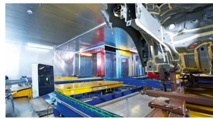
Figure 1: Car body identification with RFU630 UHF write/read device and temperature-resistant UHF label attached directly to the body
