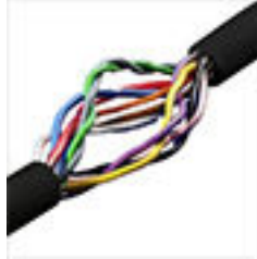
Figure 1: Twisted pair signal lines
