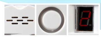
Power connected, the power indicator(green) is constantly on, and it alarms with beep sound(alarm indicator flashes twice). The digital tube displays "-" and about 4 minutes displays concentration, then it starts the alarm detection mode.
