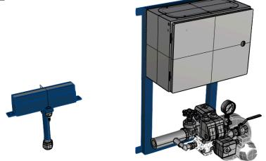
LN – Nido d'ape solution is developed according to the customer needs. It's equipped with mixer with gas train, blower and all necessary devices. The control unit is placed inside the panel and Bruciatori Santin can also supply special support for an easy installation.
