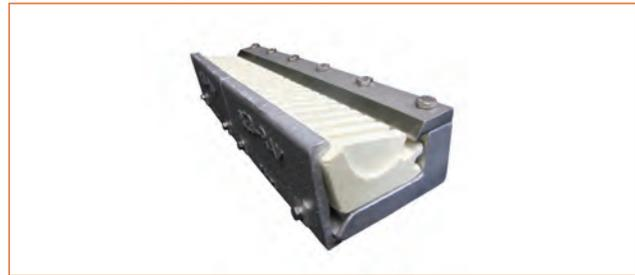
The F-SS-SC is a 12" burner with high temperature, corrosion-resistant alloy side plates and a machined stainless steel baffle plate. The smooth edge of the baffle plate promotes a uniform air/gas flow through the slit orifice, which optimizes the combustion process. The FH-SS-SC is a 7" burner with alloy side and baffle plates. Their corrosion resistance and ability to withstand high temperatures make these two models ideal choices for food applications, such as tortilla chip ovens.
