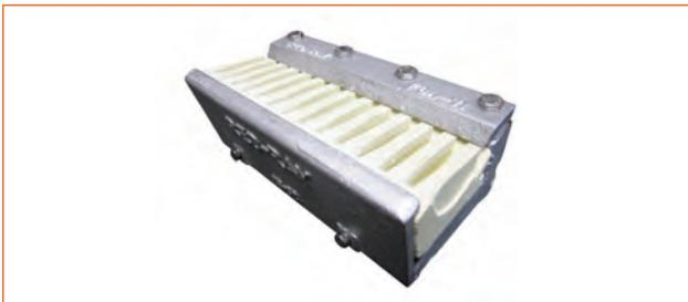
layers surrounding a part. The air-gas mixture travels from the manifold through the body of the burner and is directed onto the refractory through a slit orifice along the length of the burner. The slit orifice design optimizes the life and performance of the burner since it promotes a smooth, consistent flow of gas and is not prone to particulate build-up or clogging as are other designs, such as ported orifices.
