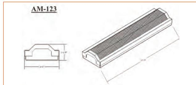
The maximum 5" diameter design of the entire burner allows retrofitting into the existing ribbon burner ports of commercial baking ovens without any modifications. We have designed the AM series to adapt to a flanged assembly, which is typically bolted to the outside of an oven wall. This design accommodates the threaded stainless steel pipe manifold inlet and the insulated ignitor/monitor assembly by extending these both through the cast iron flange on the outside of the oven wall.
