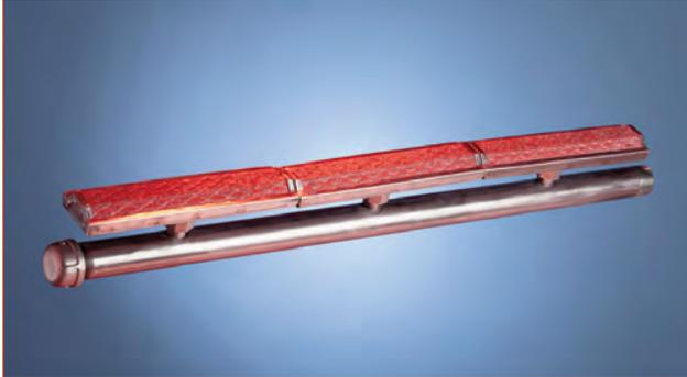
**The Apollo-Ray angled media (AM) burner model is a surface combustion gas-fired infrared burner. The emitter's symmetrical trapezoid shape allows the radiation from the angled emitter to spread over a 135° radius.**
