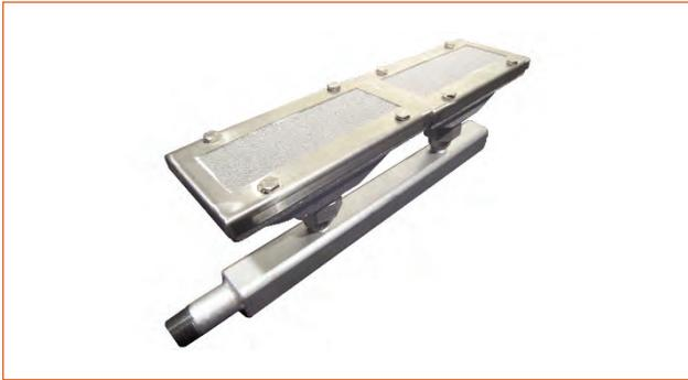
**The MR-7 is a compact atmospheric infrared burner (7.0"x3.625") that can be fed with an inspirator mixer (atmospheric) as opposed to an aspirator mixer (premix). It is a surface combustion burner that generates low heat flux infrared radiation.**
