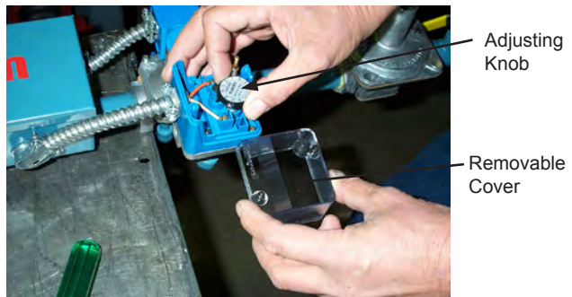
Figure E-8 Gas Pressure Switch Adjustment
