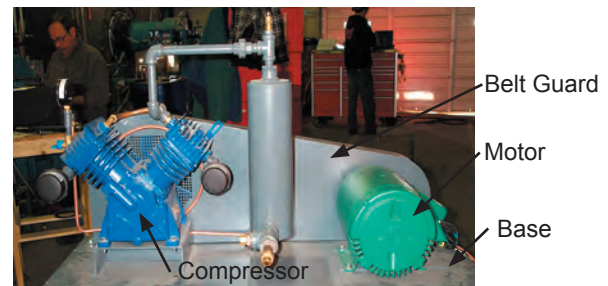
Figure B-21 Small Air Compressor
