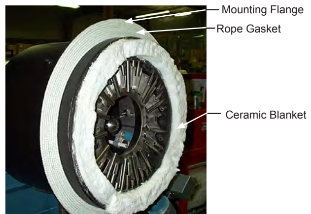
Figure B-13 Gas Manifold
