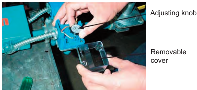
Figure E-4 Gas Pressure Switch Adjustment
