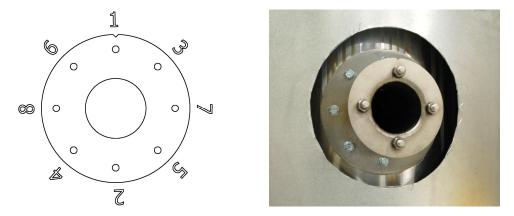
Figure 9: Fastening Order & Collector Installed
