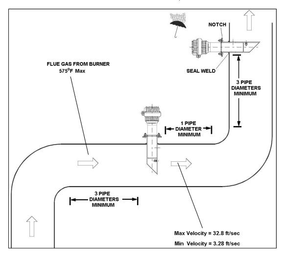
**Figure 2: Mounting Location Guide**
