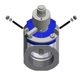
Figure 4: Mechanical Stop Installation
