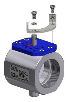
Figure 2: Mechanical Stop Bracket Installation
