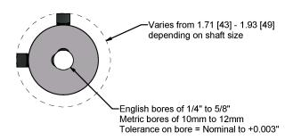
\*If mounting coupling on a 5/16" round valve / damper shaft, minimum shaft engagement is 0.50 [13]
