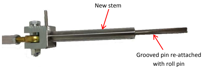
Figure 4: Reassembled Stem and Pin
