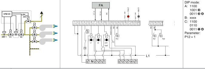
Valve check via pilot valves, venting to V2 via LGV<sub>type2 (normally closed)</sub> into the burner chamber Valve check system component: VPM-VC, Pp, LGV<sub>Type2</sub> (NC)
