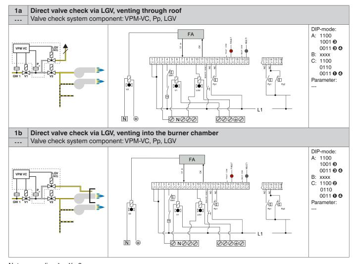
Notes regarding 1a, 1b, 2: If a valve closed when not powered is replaced instead of a LGV (open when not powered), it must be connected to output V2 (terminal 8).
