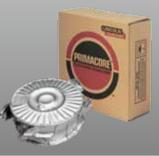
PRIMACORE™ LW-75 is a basic type, mixed gas shielded flux-cored welding wire designed for all-position welding of mild steel in applications requiring excellent hot and cold crack resistance and high impact toughness values. PRIMACORE™ LW-75 produces very low diffusible hydrogen and good weldability including vertical up. DC- polarity is recommended to use for welding in all positions.
