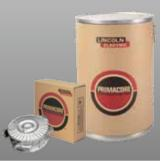
PRIMACORE™ LW-81K2 is a basic-rutile, micro-alloyed, CO₂ shielded flux-cored welding wire designed for all-position welding of mild steel and 550Mpa grade high tensile strength steel in applications requiring consistently high impact toughness values. PRIMACORE™ LW-81K2 provides excellent bead appearance and operating characteristics.
