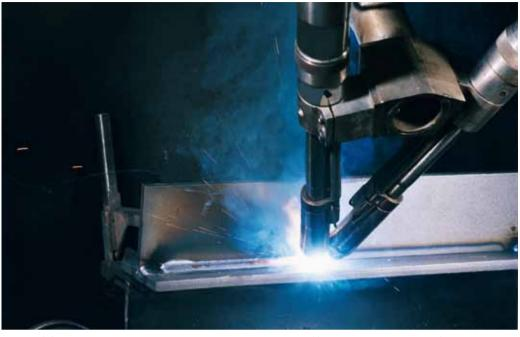
PRIMACORE™ LW-81Ni1 is an all position gas shielded 1% Nickel, micro alloyed flux-cored welding wire. It is designed specifically for applications where exceptional low temperature impact properties are required.
