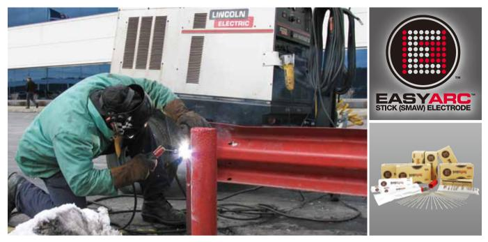
EASYARC™ 7018-1H4R is an iron powder low-hydrogen type electrode for all-position welding of mild and low alloy steels. The strictly controlled diffusible hydrogen and moisture of EASYARC™ 7018-1H4R makes it well suited for critical welding applications that require excellent cracking resistance. EASYARC™ 7018-1H4R offers superb mechanical properties, notch toughness and high efficiency at low temperature.
