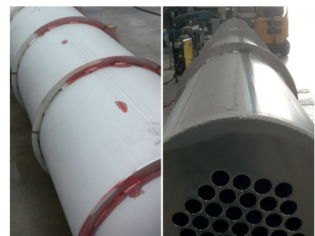
Photos showing the application of RedOne™ Pickling Paste and pickling at low temperature (+8 °C) of high alloyed heat exchanger 2205 (1.4462)
