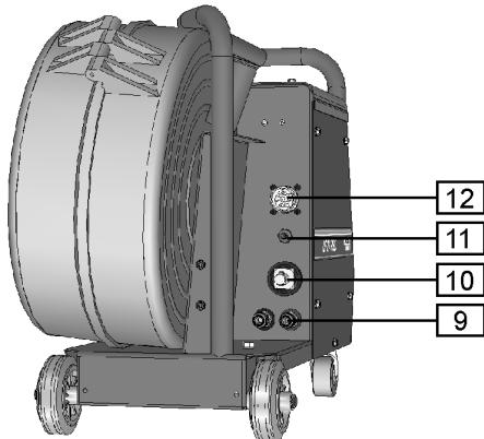
9. **Quick Connect Couplings (For water cooled model only):** If water cooled torches are used, connect water lines from water cooler here. Refer to torch and water cooler guidelines for recommended cooling liquid and flow rates.
