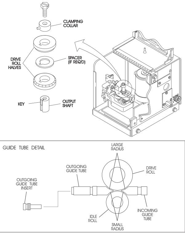
FIGURE B.2 – INSTALLING DRIVE ROLLS ON A TWO-ROLL FEEDER.
