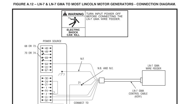
N.A. WELDING CABLES MUST BE OF PROPER CAPACITY FOR THE CURRENT AND DUTY CYCLE OF IMMEDIATE AND FUTURE APPLICATIONS.
