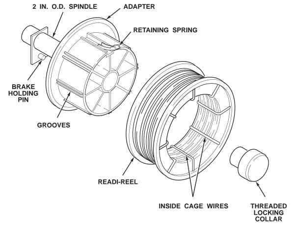
FIGURE B.5 - INSTALLING A 30 LB READI-REEL PACKAGE.
