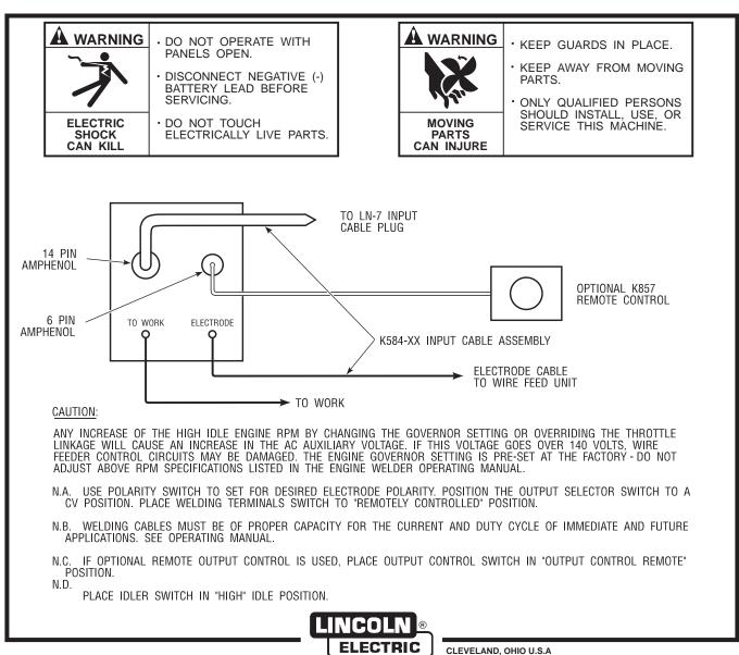
FIGURE A.15 - LN-7 & LN-7 GMA TO RANGER 10-LX - CONNECTION DIAGRAM.
