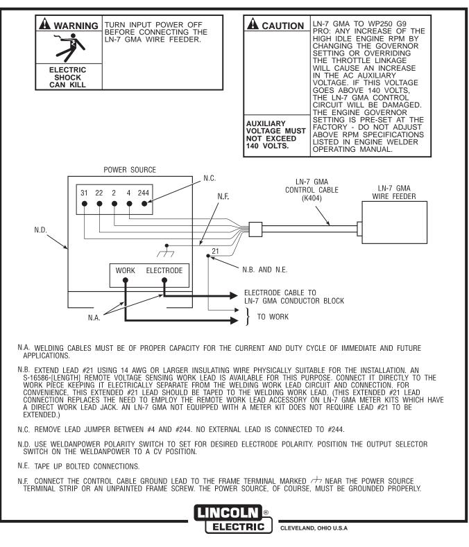
FIGURE A.14 - LN-7 & LN-7 GMA TO RANGER 9 - CONNECTION DIAGRAM.
