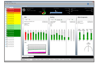
Transformer health/risk overview
