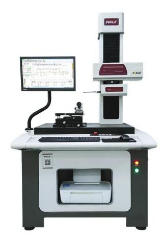
Cost-effective roughness and contour one time measurement solution. Adopt high rigidity, high accuracy, maintenance-free linear motion guide rail, can control the measuring system with high precision performance.
